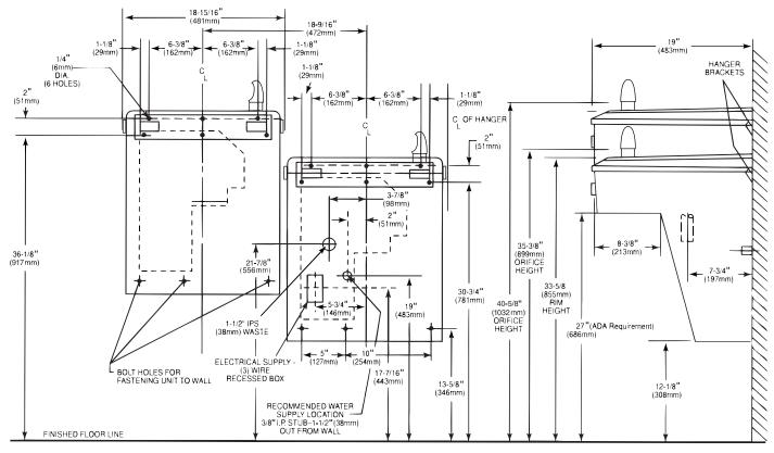
NOTE: A service supply stop should be installed at the cooler inlet tube
