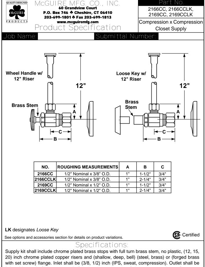
(3/8, 1/2) inch (IPS, compression). Supply kit shall equal McGuire\_\_\_\_\_\_. Supply kit shall be certified by CSA or other recognized testing authority and bear manufacturer and testing mark.
