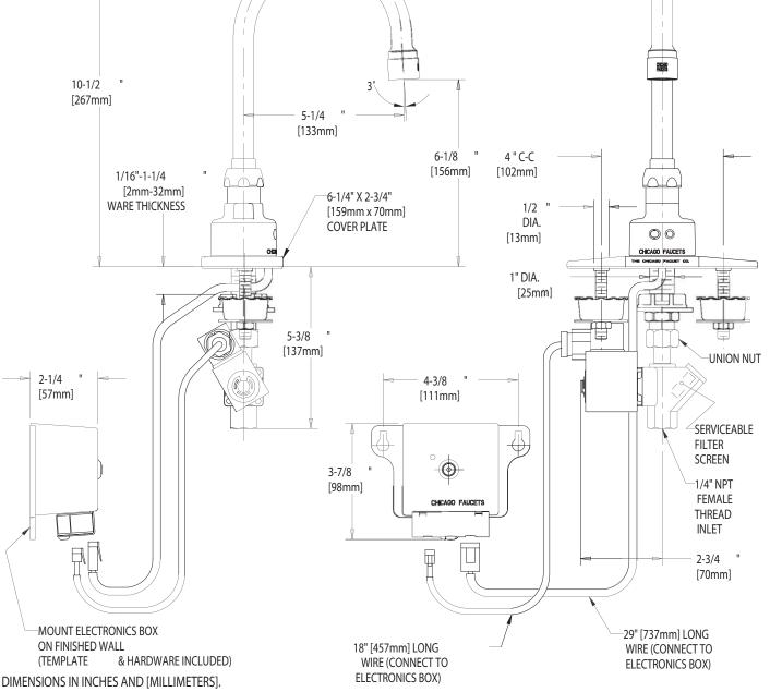
**TECHNICAL DATA** DATE: 05-01-02 - 4" C-C ELECTRONIC SINK FITTING - 0.5 GPM (1.9 L/min) VANDAL BY: SID WITH INFRARED SENSOR RESISTANT SPRAY OUTLET CHK'D: - FORGED BRASS SPOUT BASE AND COVER PLATE - INCLUDES OPTIONAL 2.2 GPM - GN2AH8 GOOSENECK SPOUT (8.3 L/min) AERATOR INSERT - 6 VOLT D/C POWER REQUIRED. - CHROME PLATE FINISH APP'D:
