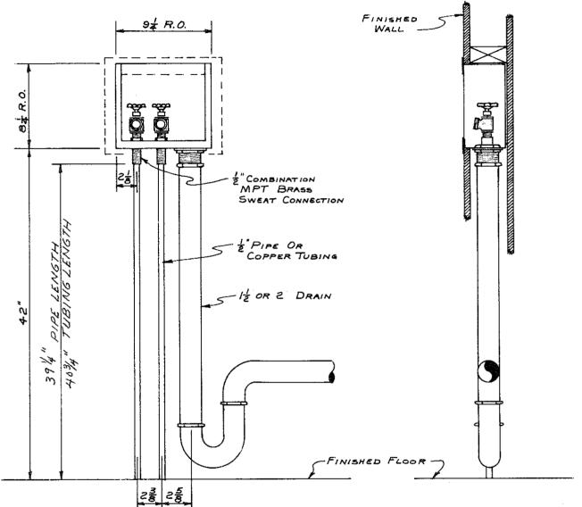
PLUMBING ROUGHING-IN MEASUREMENTS FOR SPACE SAVER WASHING MACHINE SUPPLY AND DRAIN MODEL FB 150 & FB 200
