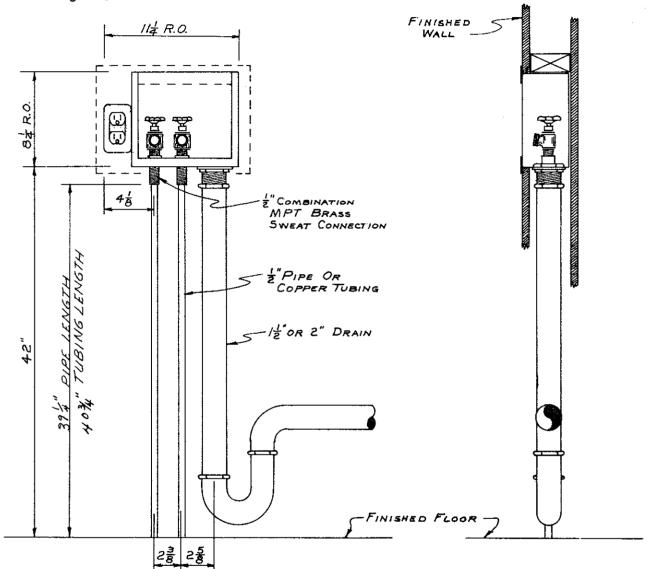
PLUMBING ROUGHING-IN MEASUREMENTS FOR SPACE SAVER WASHING MACHINE SUPPLY AND DRAIN MODEL FBE 150 & FBE 200
