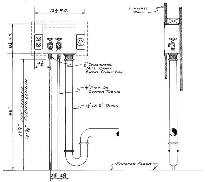
PLUMBING ROUGHING-IN MEASUREMENTS FOR SPACE SAVER WASHING MACHINE SUPPLY AND DRAIN MODEL FBED 150 & FBED 200
