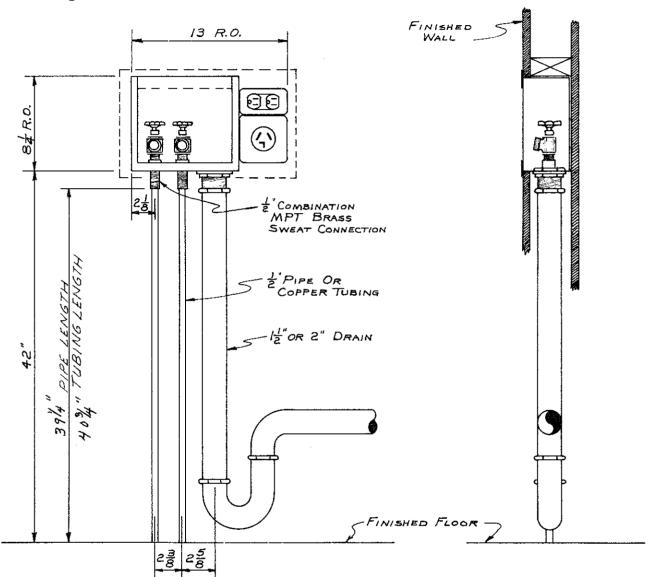
PLUMBING ROUGHING-IN MEASUREMENTS FOR SPACE SAVER WASHING MACHINE SUPPLY AND DRAIN MODEL FNWBED 150 & FNWBED 200
