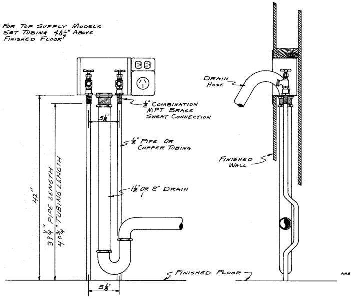
PLUMBING ROUGHING-IN MEASUREMENTS FOR SPACE SAVER WASHING MACHINE SUPPLY AND DRAIN - MODEL NWBED-150 & NWBED-200
