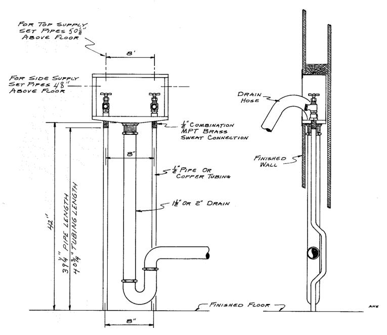
PLUMBING ROUGHING-IN MEASUREMENTS FOR SPACE SAVER
