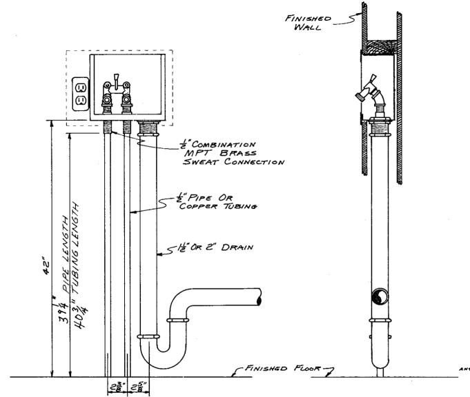
PLUMBING ROUGHING-IN MEASUREMENTS FOR SPACE SAVER WASHING MACHINE SUPPLY AND DRAIN MODEL WBE 150 & WBE 200
