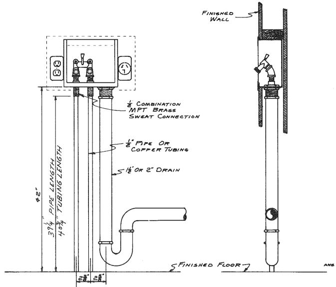
PLUMBING ROUGHING-IN MEASUREMENTS FOR SPACE SAVER WASHING
