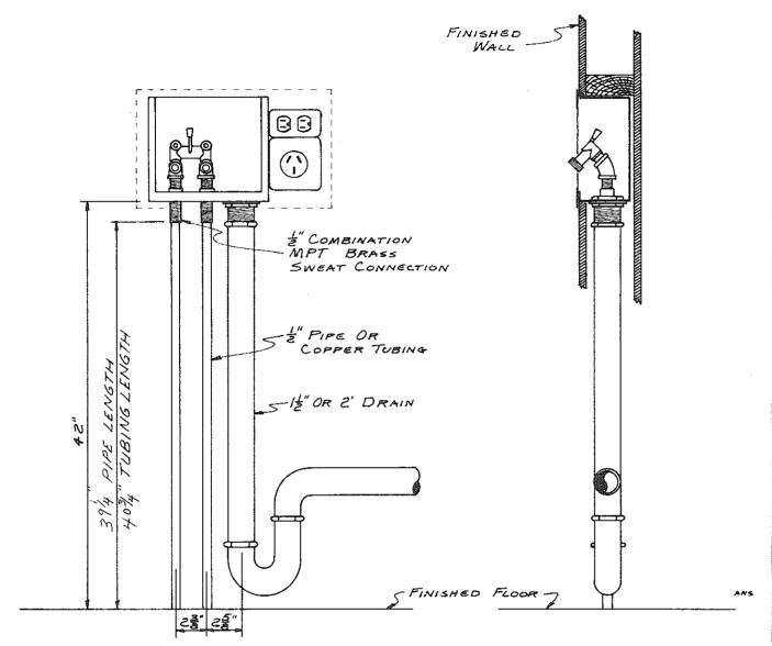
PLUMBING ROUGHING-IN MEASUREMENTS FOR SPACE SAVER WASHING MACHINE SUPPLY AND DRAIN MODEL WNWBED 150 \$ WNWBED 200
