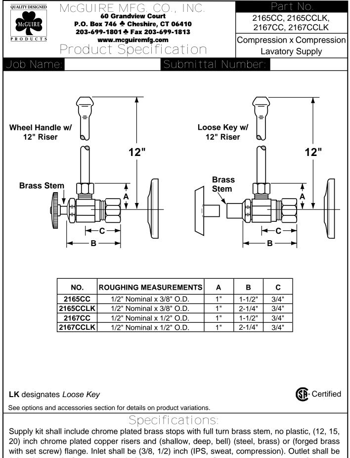
(3/8, 1/2) inch (IPS, compression). Supply kit shall be McGuire \_\_\_\_\_\_. Supply kit shall be certified by CSA or other recognized testing authority and bear manufacturer and testing mark. Stop to be certified to 200 psi line pressure.
