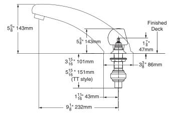
Standard rough-in adjusts up to 1-3/8" maximum deck thickness. For 2" additional adjustment use S-247-TT-BDY or S-247-1-TT-BDY.
