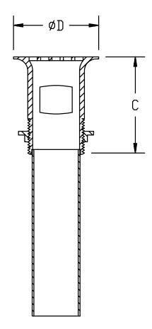
**Engineering Specification:** Zurn Z8743 – Cast brass solid top, open grid, P.O. plug with 5[127] 17 gauge tailpiece and cast brass locknut for sink depth up to 2 1/4[57]. 6-, 8-, 10- and 12- tailpieces available.
